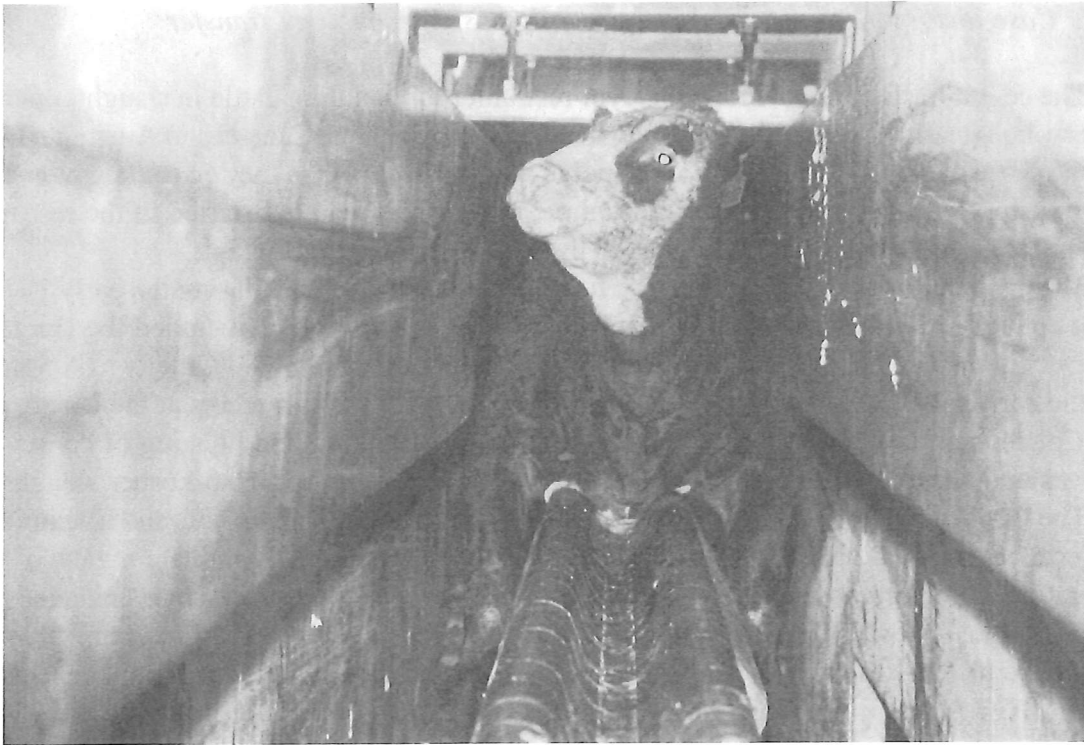
Fig. 1. A steer sits quietly on the center track conveyor which is shaped to fit its brisket. The solid roof over the steer's head must be long enough to block his vision until his back feet are off the entrance ramp. The maximum width of the conveyor is 30 cm (reprinted from Grandin, 2000a).
